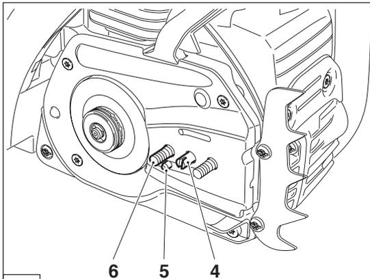
Turn chain tensioning screw (4) to the left (counter-clockwise) until the pin (5) of the chain tensioner is underneath the threaded pin (6).
