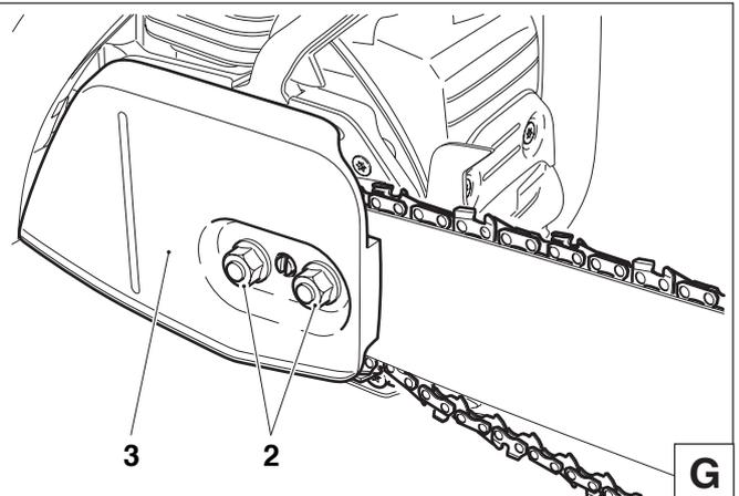
**Tightening the saw chain**
