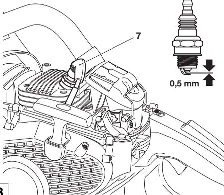
The spark plug must be replaced in case of damage to the insulator, electrode erosion (burn) or if the electrodes are very dirty or oily.
