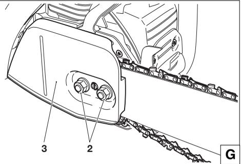
**Tightening the saw chain**
