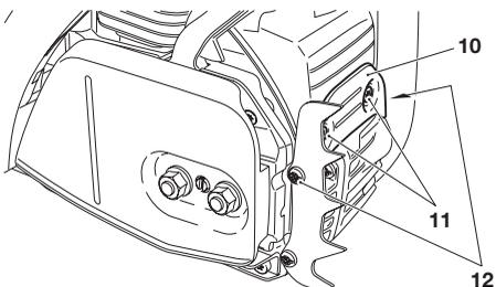
Remove the retaining plate (10) by unscrewing screws (11, short) and (12, long).
