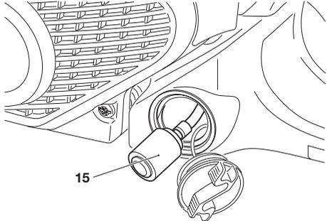
**Replacing the suction head**
