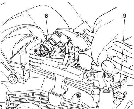
With the spark plug removed and the spark plug cap firmly seated, use insulated pliers to hold the spark plug (8) against the cylinder (not the spark plug hole).
