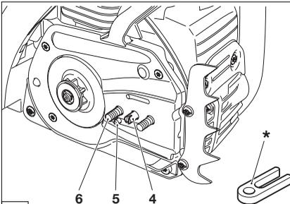
Remove the plastic transport cover (\*) and dispose of properly.
