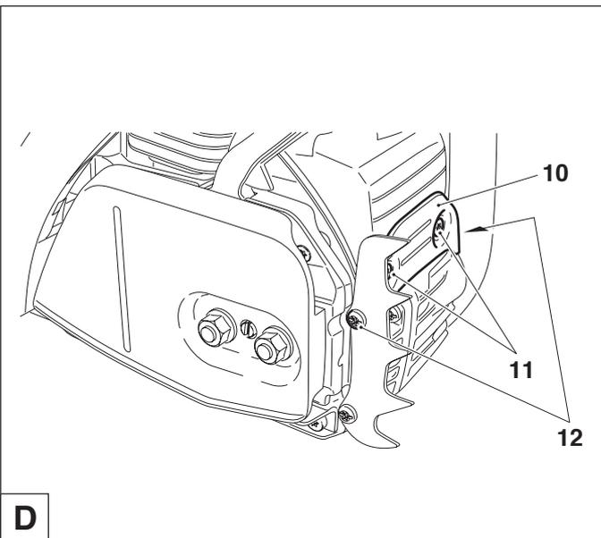
Remove the retaining plate (10) by unscrewing screws (11, short) and (12, long).
